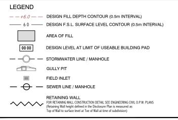
Builders shall not build off the design levels shown; a site survey is required. This note is an integral part of this plan.
