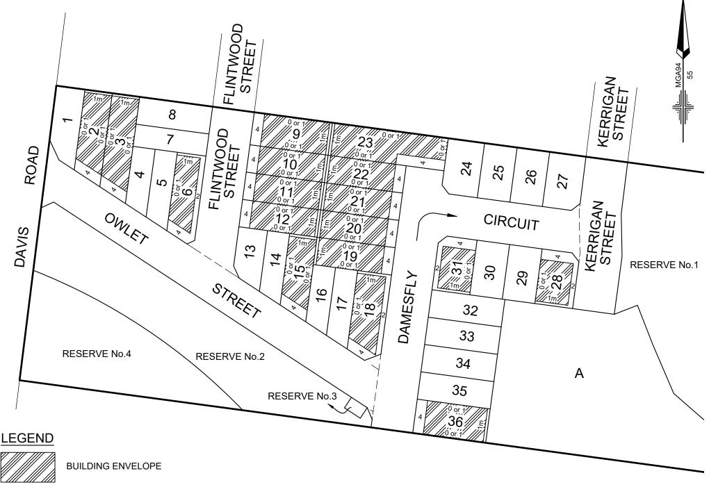
NOTE: FOR SETBACKS SHOWN "0 or 1", ONLY ONE SIDE BOUNDARY MAY BE BUILT TO WHICH ACCORDS WITH THE CROSSOVER LOCATION
